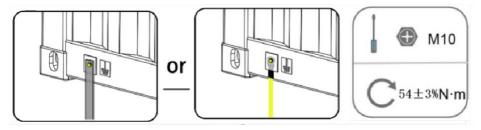
Figure 36: Schematic diagram of cabinet grounding
