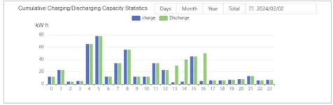
Figure 87: Cumulative charge/discharge graphs
